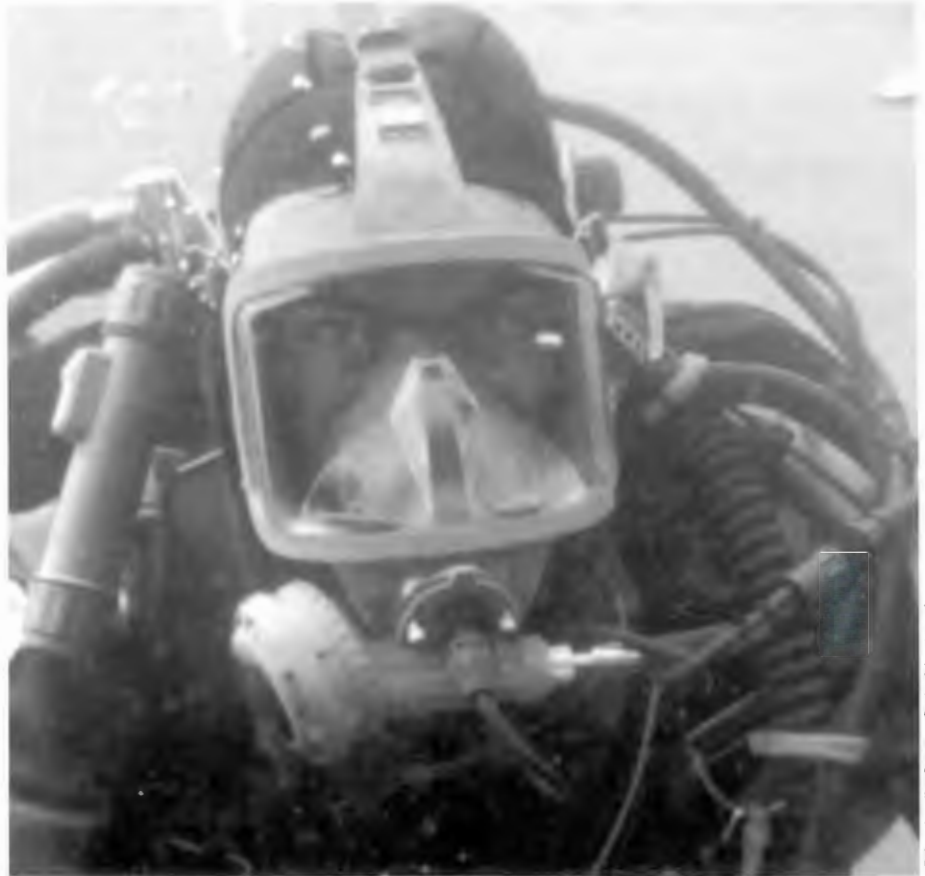
Jim Baden using the Aga full face mask with diver to diver communications.
