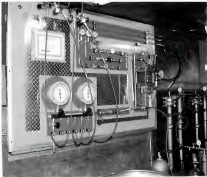
Nitrox and mixed gas blending panel at High Tech Divers Inc. in Gloucester, NJ
